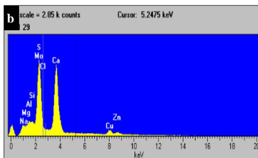
Figure (3) Shows EDX analysis of **a.** constructed sample composed of calcium, quartz, and halite, **b.** white lye sample contains calcium, sulfur, halite, and quartz.
