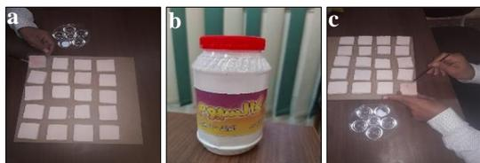
Figure (6) Shows **a.** simulation samples, **b.** calcium nano hydroxide, **c.** applying the consolidant.
