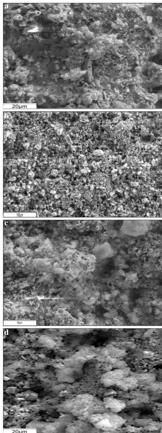
Figure (7) Shows SEM micrograph of **a.** morphology the lower layer of the Sharia Judge's tomb in the Fatimid cemetery, distribution of **b.** (2:1) nano calcium hydroxide mix with TiO<sub>2</sub> nanoparticles in treated plaster, **c.** (1:1) nano calcium hydroxide mix with TiO<sub>2</sub> nanoparticles of the treated plaster, **d.** (1:2) nano calcium hydroxide mix with TiO<sub>2</sub> nanoparticles treated plaster
